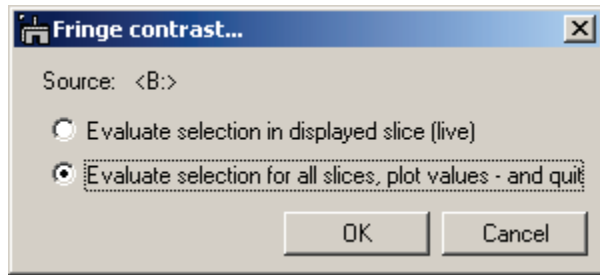
Figure 81 Computation of the fringe contrast from 3D data sets. Choose between evaluation within the selected slice or evaluate the full data set.
