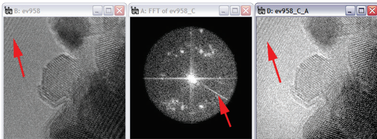
Figure 106 Left: Electron hologram exhibiting Fresnel fringes caused by the Möllenstedt biprism. Middle: The sideband exhibiting the trace of the Fresnel fringes as an artificial line. Right: Fresnel fringes appear in the reconstructed image amplitude as well.
