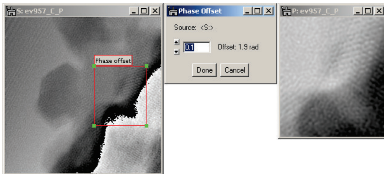
Figure 38 Phase offset allows an offset of the phase of real or complex images by a constant. If the dynamic range of the image is < 2\pi , the resulting phase will wrap automatically.
